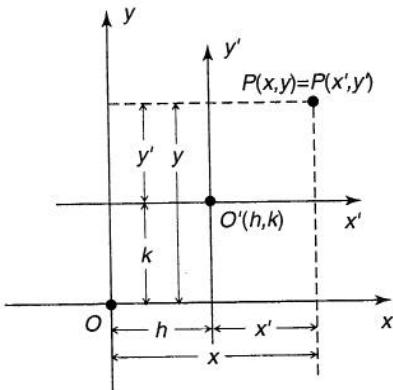
FIGURE 34 Deriving the Formulas for Translation of Axes
