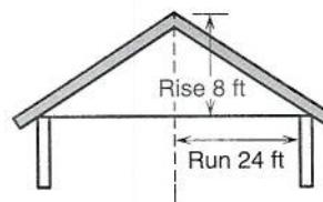
The **rise** is the increase in height and the **run** is the corresponding horizontal distance. Typically, roofers express the pitch as the amount of rise per foot, or per 12 inches, of run. Therefore, rather than write the pitch as a fraction in lowest terms, they express it as an equivalent fraction with a denominator of 12. For the roof shown,
