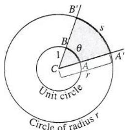
FIGURE 1.38 The radian measure of the central angle  $A'CB'$  is the number  $\theta = s/r$ . For a unit circle of radius  $r = 1$ ,  $\theta$  is the length of arc  $AB$  that central angle  $ACB$  cuts from the unit circle.
