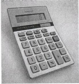
The photograph shows the **Sharp EL-330M**, a typical four-function calculator.
