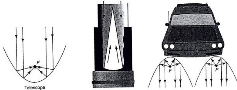
A reflecting telescope reverses the use of these same properties. Here, the rays of light from a distant star, which are nearly parallel to the axis of the parabola, are reflected by the mirror to the focus. The eyepiece is placed at the focus, where the rays of light are gathered.
